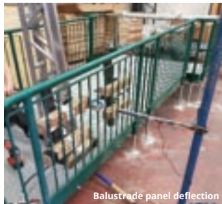
Balustrade panel deflection
