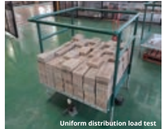
Uniform distribution load test
